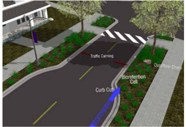
Above: Rendering of a curb bumpout along a residential street. Left: Vegetated curb extension in Portland, OR. Below: Cut-away of a curb bumpout with permeable pavers on sidewalk.
