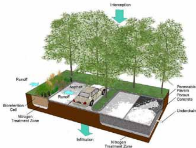
Above: Parking lot stormwater system utilizing permeable pavement, street trees, and bioretention.
